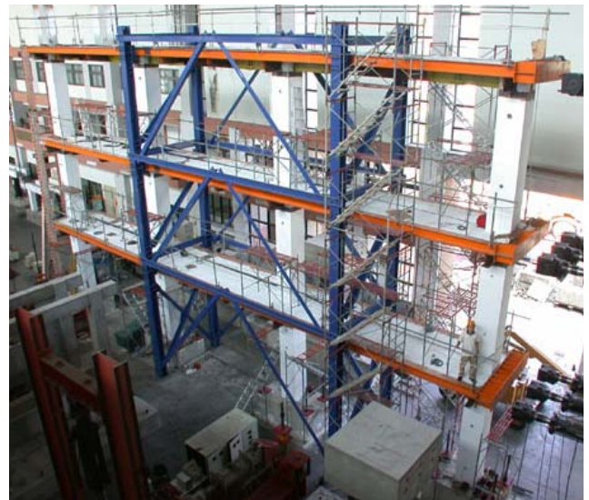
Figure 1 –Photo of full-scale composite test frame.
