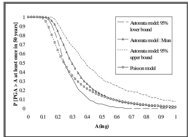
Figure 2. Site hazard curve for Palo Alto, California.
