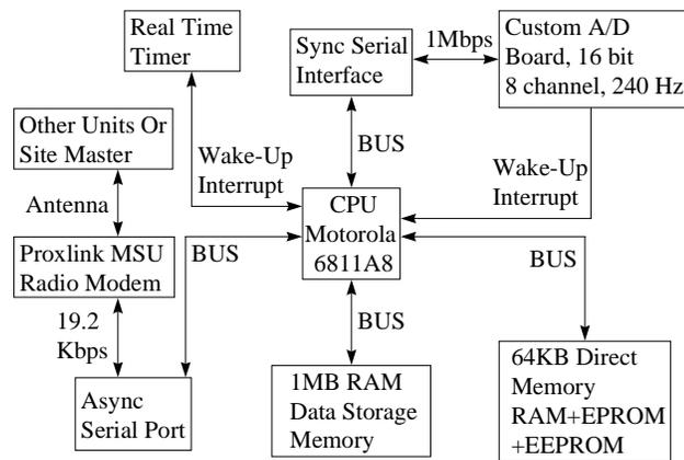
Figure 3. Sensor Unit Subsystems and Interfaces
