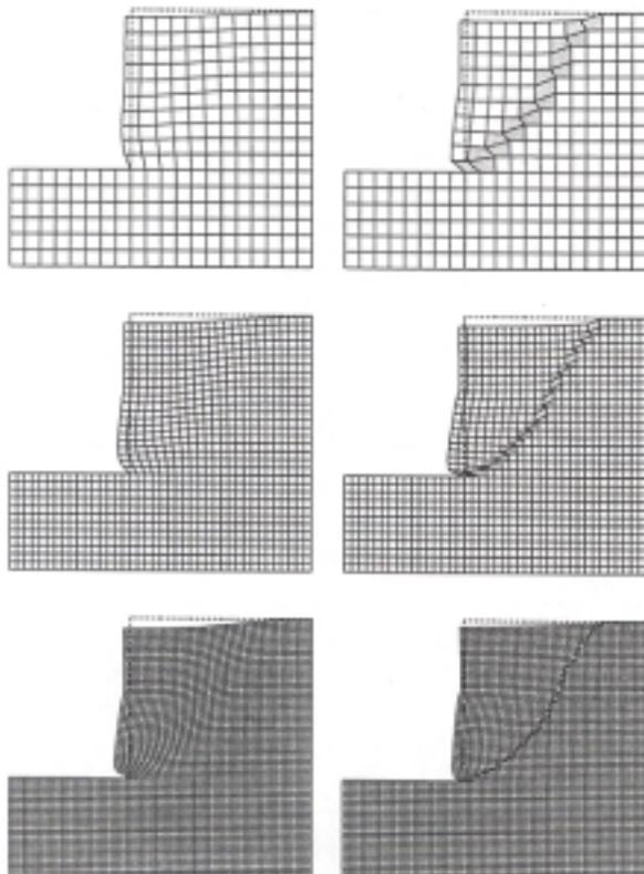
Figure 2. Deformed meshes for standard and enhanced solutions with non-associative, dilative plastic flow.
