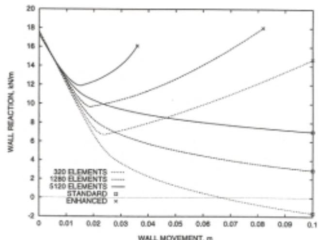
Figure 3. Load-displacement curves for non-associative, dilative plastic flow.
