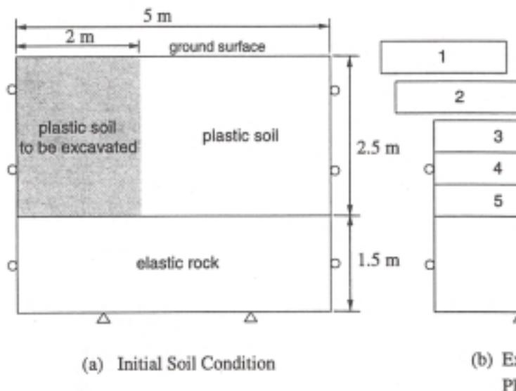
Figure 1. Plane strain excavation problem: (a) Initial soil condition showing portion of soil to be excavated. (b) Excavation sequence and placement of rigid wall showing wall reaction,  $R$ .
