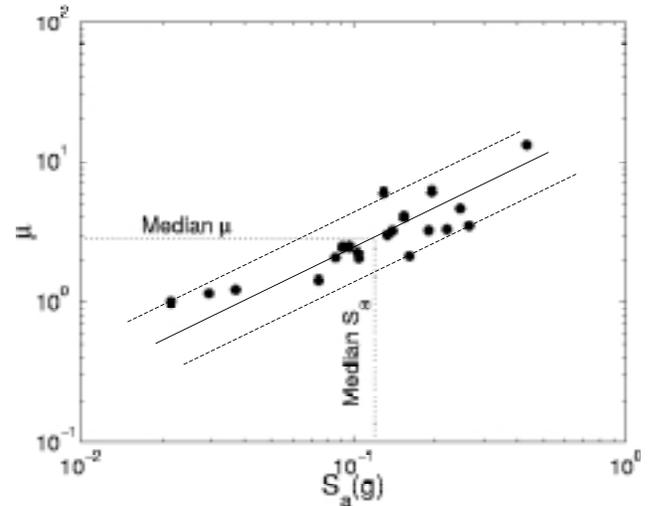
Fig. 2. Variation of drift ductility ( $\mu$ ) given  $S_a$
