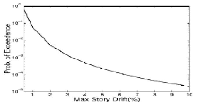
Fig. 3. PSDA curve for maximum interstory drift
