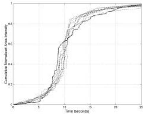
Figure 3: Cumulative normalized Arias intensity as function of time. Dashed lines: ten simulations; solid line: recording.
