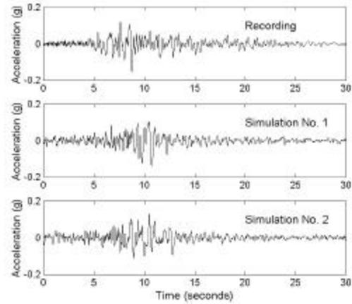
Figure 2: An example of a recorded accelerogram (top) and two simulated time histories.
