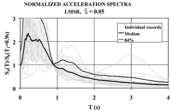
Figure 1. Set of 20 ordinary ground motions normalized to their spectral acceleration at  $T = 0.9$  seconds.
