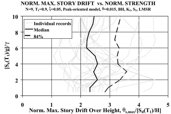
Figure 2. Maximum story drift over the height as a function of structure strength.
