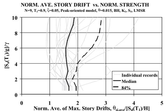
Figure 3. Average of maximum drifts in each story as a function of structure strength.
