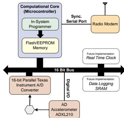
Figure 2 – Functional Layout of the Proposed Wireless Sensing Unit
