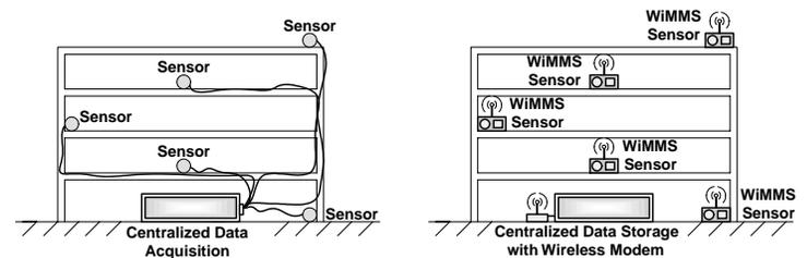
Figure 1 – Evolution from a Cable-Based to a Wireless Monitoring System
