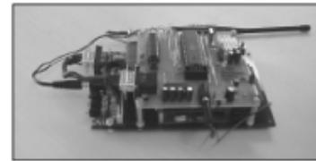
Figure 3 - Proof-of-Concept Wireless Sensing Unit
