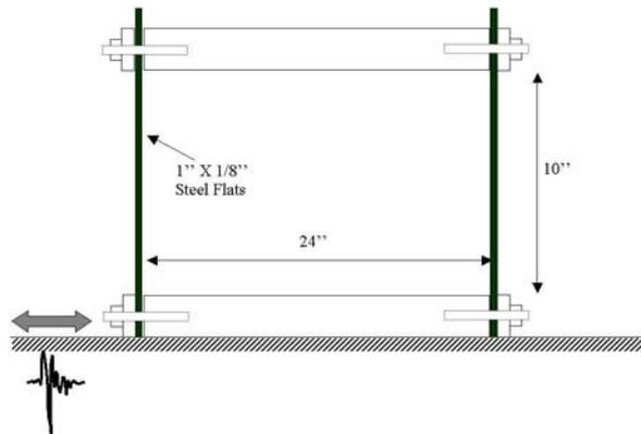
Figure 1. Schematic Elevation View of the Test Structure
