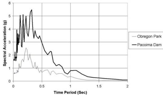
Figure 2. Response Spectra for 1% damping for both the earthquake records
