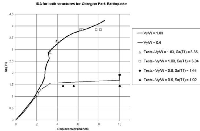
Figure 5. IDA Curves for the Obregon Park Record (both structures)
