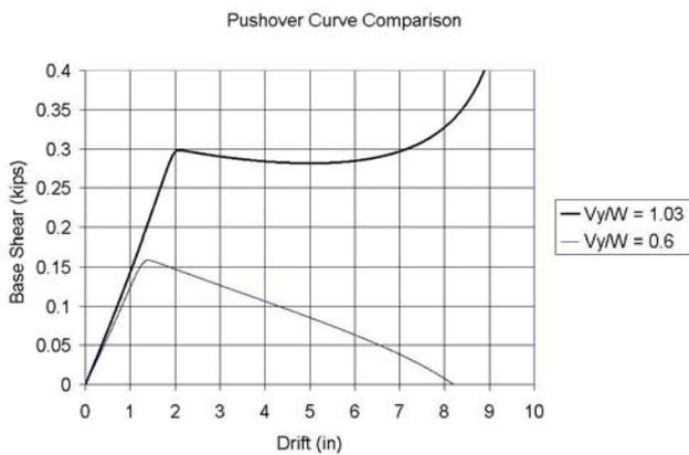
Figure 4. Pushover curves for both the structures
