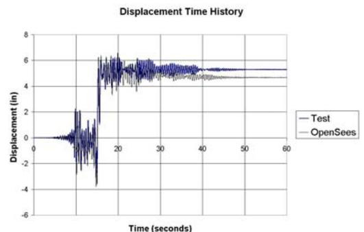
Figure 3. Displacement Time History Comparison between Test and Analysis
