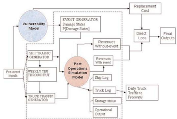
Figure 1. Components of the loss estimation methodology.
