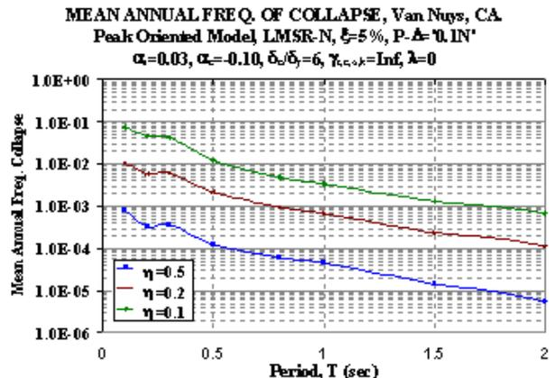
Figure 5 Mean Annual Frequency of Collapse for SDOF systems
