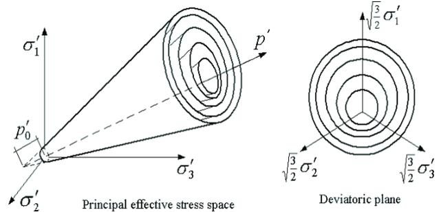
Figure 1 - Conical yield surface in principal stress space and deviatoric plane
