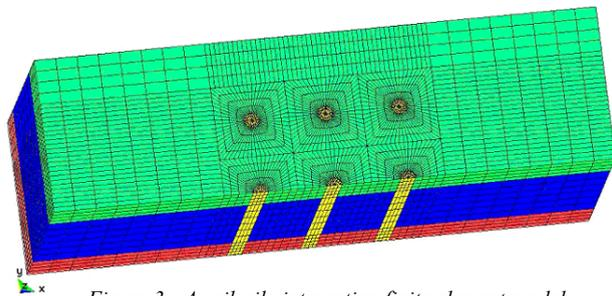
Figure 3 - A soil-pile interaction finite element model
