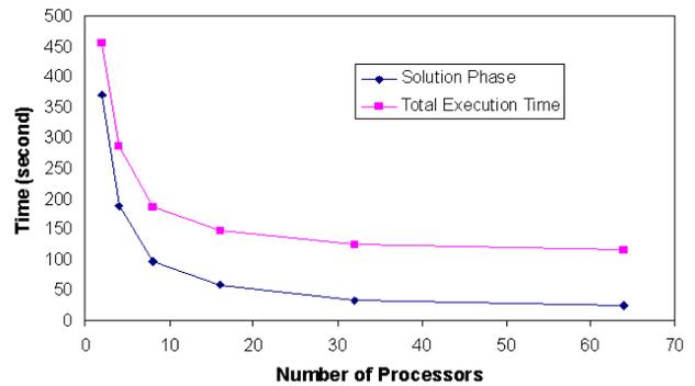
Figure 4 - Solution times for the soil-pile interaction method
