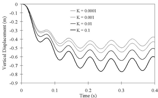
Figure 2. Finite deformation analysis: vertical displacements of node A with hydraulic conductivity varying from 0.1 m/s to 0.0001 m/s.
