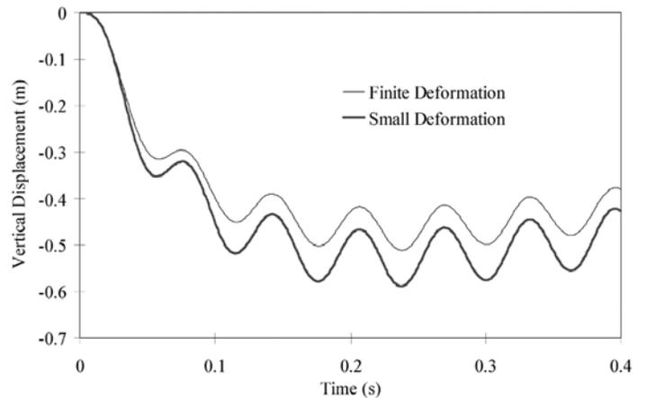
Figure 3. Comparison of vertical displacement of node A between the small and finite deformation analyses with  $K = 0.0001$  m/s.
