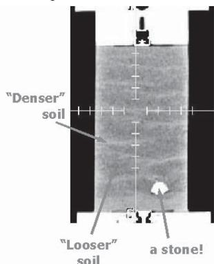
*X-ray computer tomography (X-ray CT) scan of a soil specimen for input into a strain localization finite element model.*
