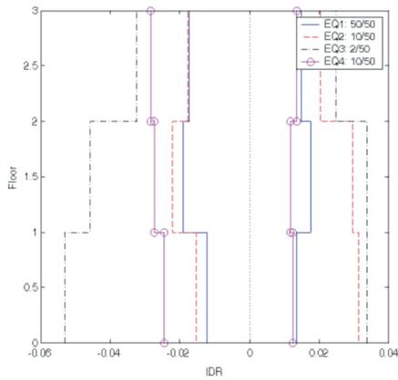
Figure 3 - Max/Min Drifts during EQ
