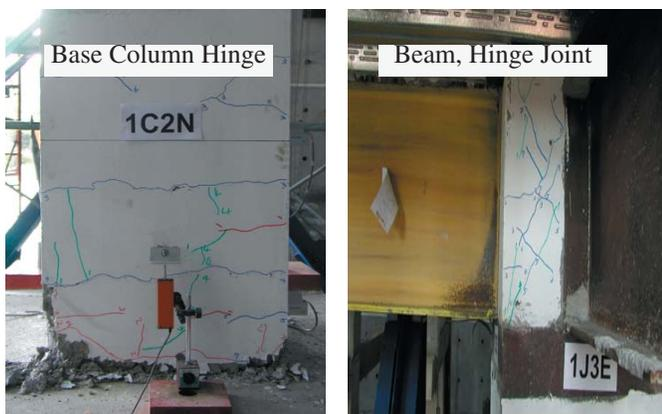
Figure 4 - Typical Damage after Design Event
