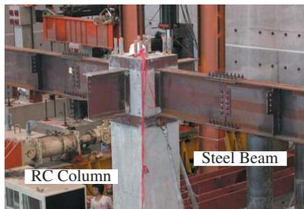
Figure 1 - Typical Composite Joint
