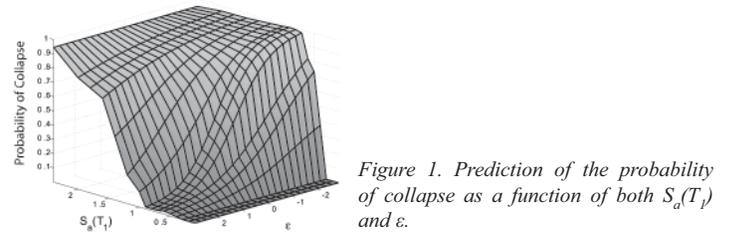
Figure 1. Prediction of the probability of collapse as a function of both  $S_a(T_1)$  and  $\epsilon$ .
