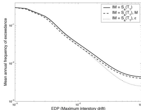
Figure 3. Mean annual frequency of exceedance versus maximum interstory drift using scalar and vector-valued  $IM$ s.
