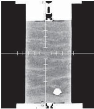
Figure 1: Cross-section through a biaxial test specimen of silica sand; white spot is a piece of gravel
