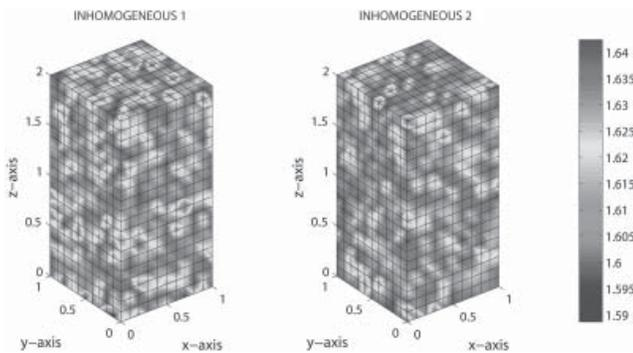
Figure 2: Initial specific volume field and finite element discretization for inhomogeneous rectangular specimens
