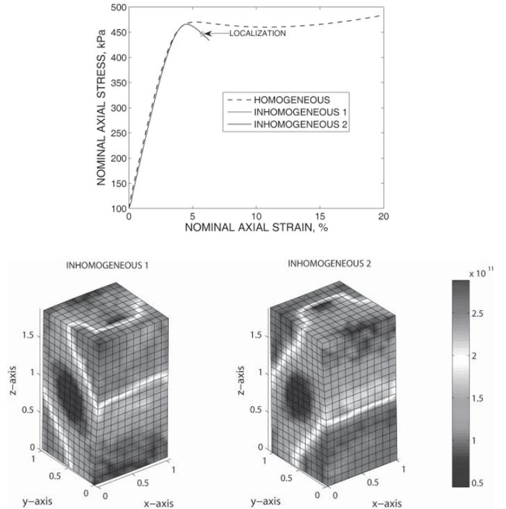
Figure 4: Contour of determinant function at onset of localization for inhomogeneous rectangular specimens
