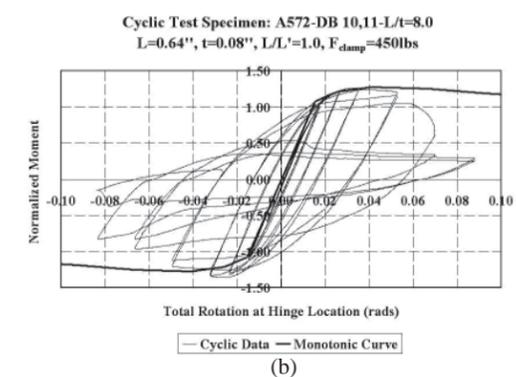
Figure 3: (a) Clamped specimens to control early local buckling gages attached on the steel plates, (b) cyclic behavior of plastic hinge region with length to thickness of reduced section equal to 8
