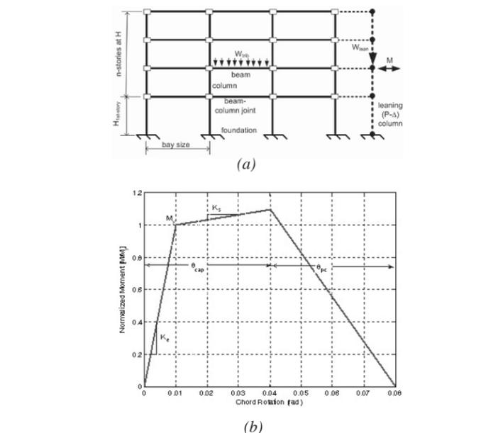
Figure 1. Analytical model for frame structures, showing (a) generalized 2D model configuration and (b) nonlinear material features of beam-column hinges.
