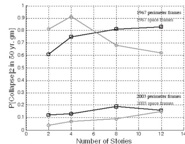
Figure 4. Predicted collapse performance of code-conforming (2003) and existing (1967) reinforced concrete moment frames. Due to changes in building code provisions, particularly related to reinforcement detailing and capacity design, the 2003 structures are much safer.
