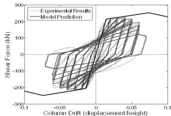
Figure 2. Calibration of RC beam-column model to experimental test by Saatcioglu and Grira (1999) [specimen BG-6].
