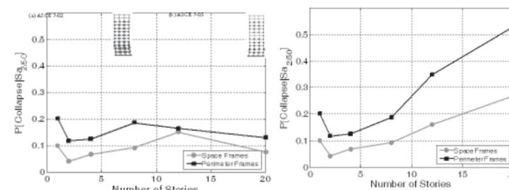
Figure 3. Predicted collapse performance of reinforced concrete special moment frames, measured in terms of probability of collapse for a 2% in 50 year ground motion. Comparison of figures (a) and (b) illustrates the minimum base shear requirements change between ASCE 7-02 and ASCE 7-05. The building images show the predominant collapse mechanism for the 12-story structure, which is more localized for the weaker ASCE 7-05 designs.
