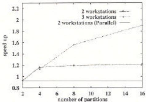
(b) Example Run on Distributed Workstations (with one work-station loaded)
