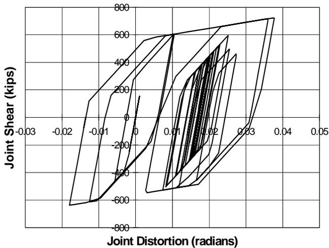
Figure 3. Joint Shear-Distortion Response
