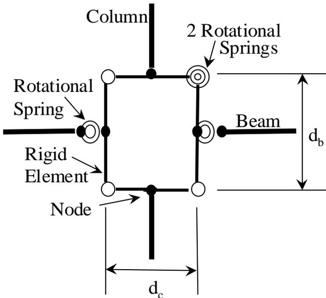
Figure 2. Analytical Model of Joint Panel Zone
